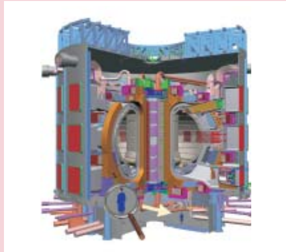
Cut-away drawing of the ITER tokamak showing the D-shaped vacuum vessel, surrounding structures, and the cylindrical cryostat which forms one of several safety barriers.
